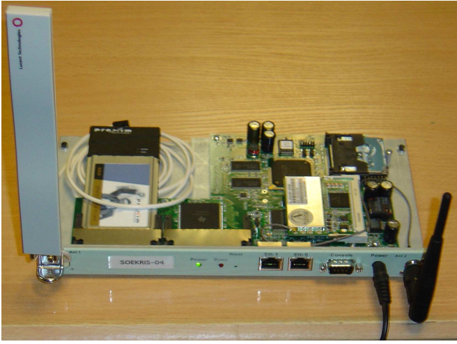
Fig. 2. MeshDVBox: the custom wireless mesh router used to build the MeshDVNet testbed.
