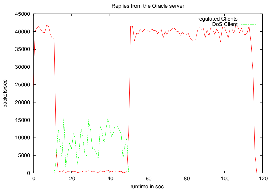
Figure 21: replies from an Oracle server to regulated and flooding clients
