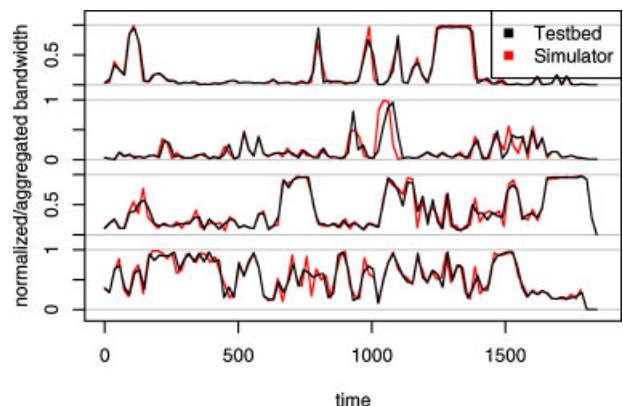
Figure 2. Link utilisation in terms of normalised bandwidth usage for both a simulator and a testbed run for one of the trace-based experiments and direct routing.
