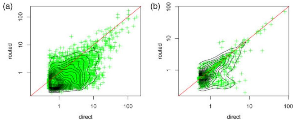
Figure 6. Scatter plots of flow durations with and without routing for the MWN traces and the `MinLargeFlows` strategy. In addition, a contour plot is superimposed. (a) Full MWN trace; (b) 1/3MWN trace.
