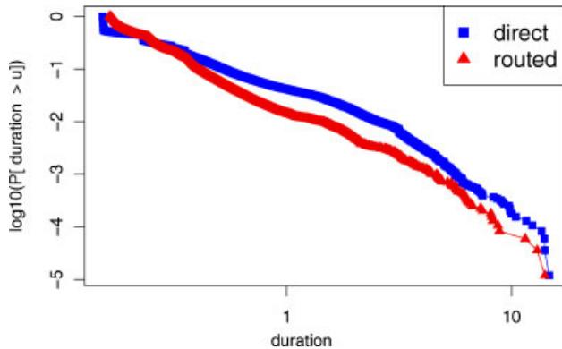
Figure 3. CCDF of flow durations with and without routing for the Surge Web workload and the MinLargeFlows strategy.
