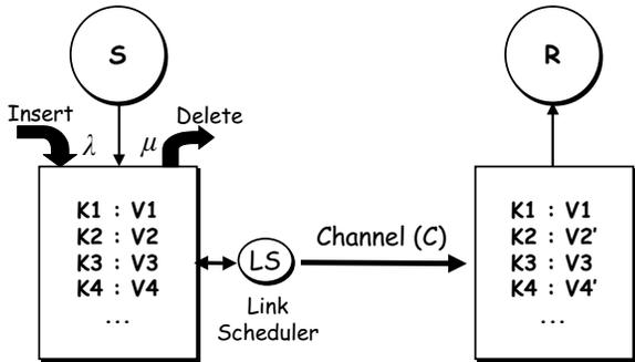
Figure 1: Soft state data model comprises an evolving table of  $\{key, value\}$  pairs.
