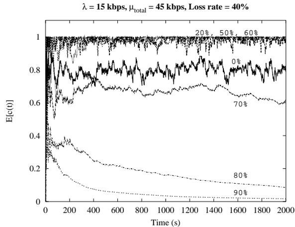
Figure 8: In open-loop ( $\mu_{fb}/\mu_{tot} = 0$ ), consistency is about 80%. When  $\mu_{fb}/\mu_{tot} = 20 - 60\%$ , consistency reaches 99%. At higher values, when insufficient bandwidth is available for data, consistency collapses.
