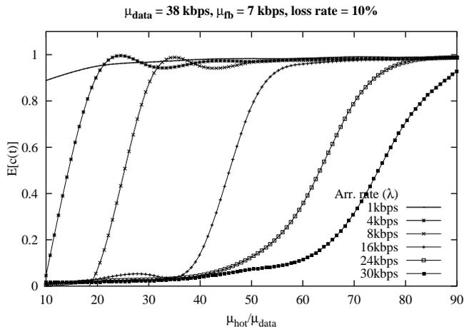
Figure 10:  $\lambda \leq \mu_{hot}$  is the optimal region beyond which the marginal benefit from additional bandwidth to the “hot” queue is limited and below which system consistency shows marked degradation.
