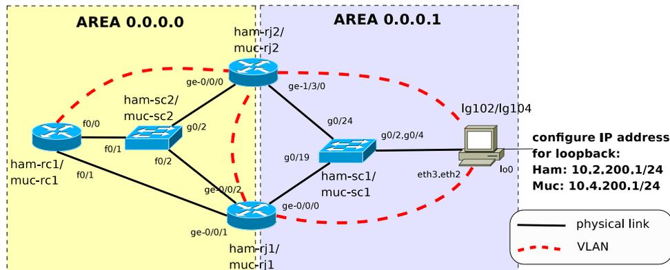
Figure 1: Topology – Basic Configuration.
